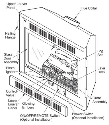
Figure 1 - Direct-Vent Fireplace with Millivolt Ignition
